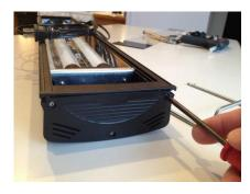
5. Remove bulbs, then remove screws securing bulb holder assembly; slide assembly out.
