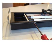
4. Turn bulb end caps counter-clockwise to loosen and pull back caps, spacers and washers.
