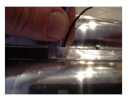
Make sure polarity is correct.All LEDs must be plugged in correctly to light.
