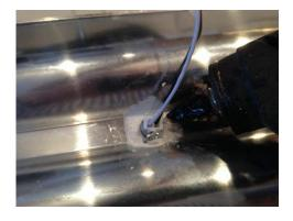
10. Insert white socket into clear holder from back of reflector.
