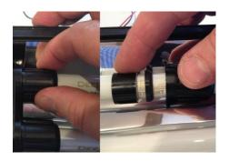
6. Slide out reflector, disconnect LED power. plug from socket.
