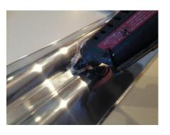
2. Loosen screws on support leg farthest from cord and remove leg.
