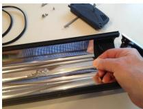
8. Push clear LED holder into hole through front of reflector.
