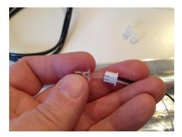
11. Install LED into socket.
