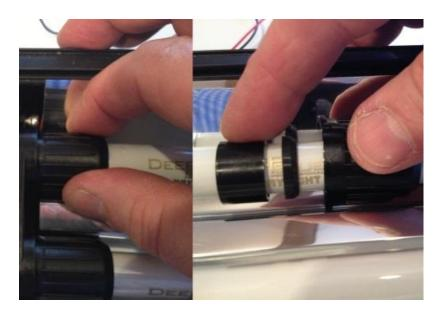
3. Slide plastic parts off old bulb and reinstall on new bulb in the same positions. Slide new bulb into slots and rotate until you feel it 'click' into place. Slide caps, spacers and washers back into place and tighten, then slide lens back into fixture.
