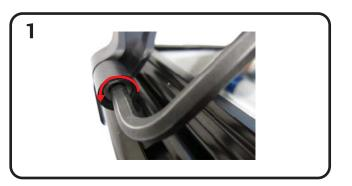
1.) IF THE MOUNTING LEGS ARE INSTALLED, USE A 5MM HEX DRIVER AND REMOVE THE MOUNTING LEGS BY TURNING COUNTER CLOCKWISE. PLEASE SEE FIGURE 1 ON THE LEFT.
